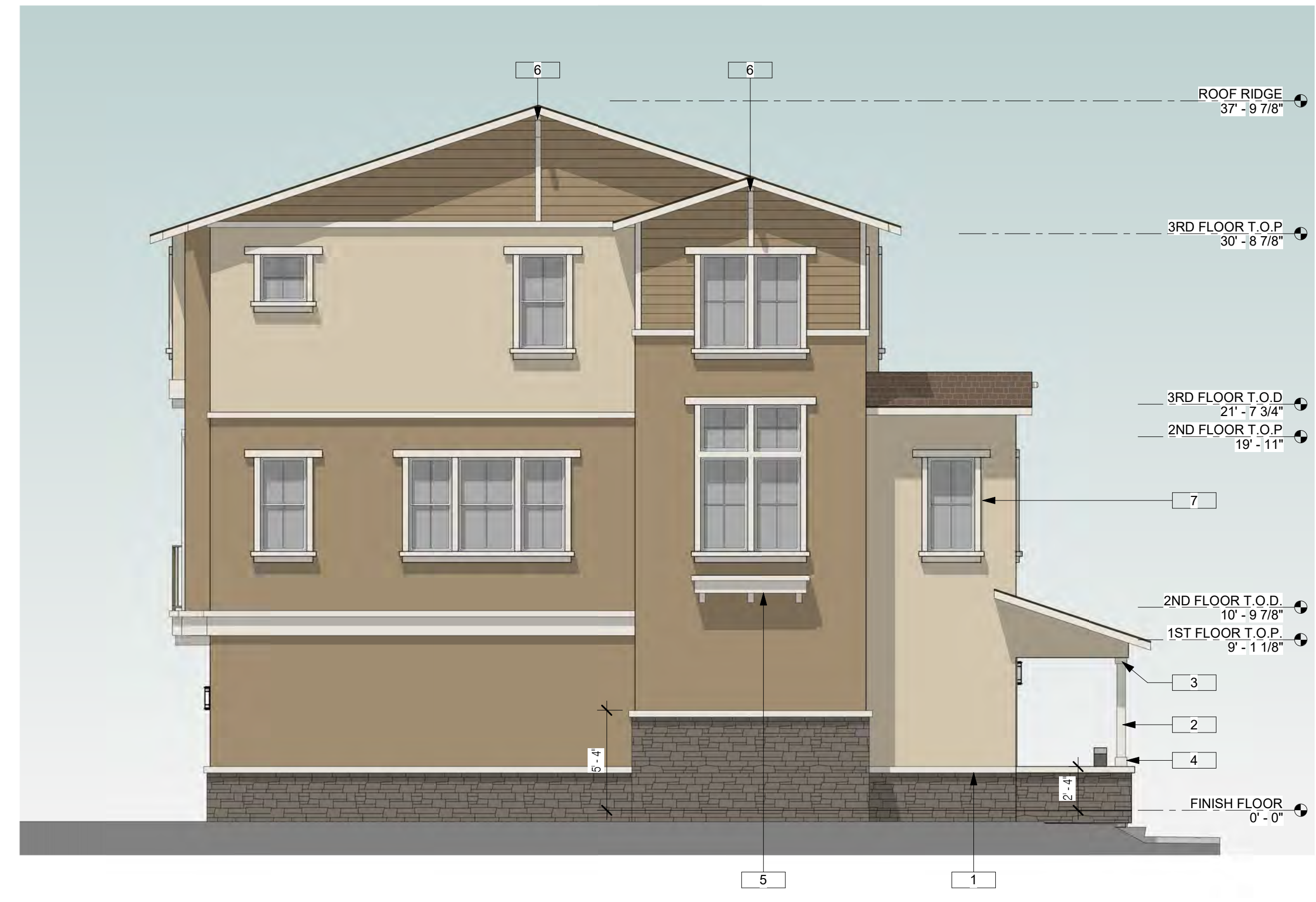
1 EXTERIOR ELEVATION A - REAR 3/16" = 1'-0"
