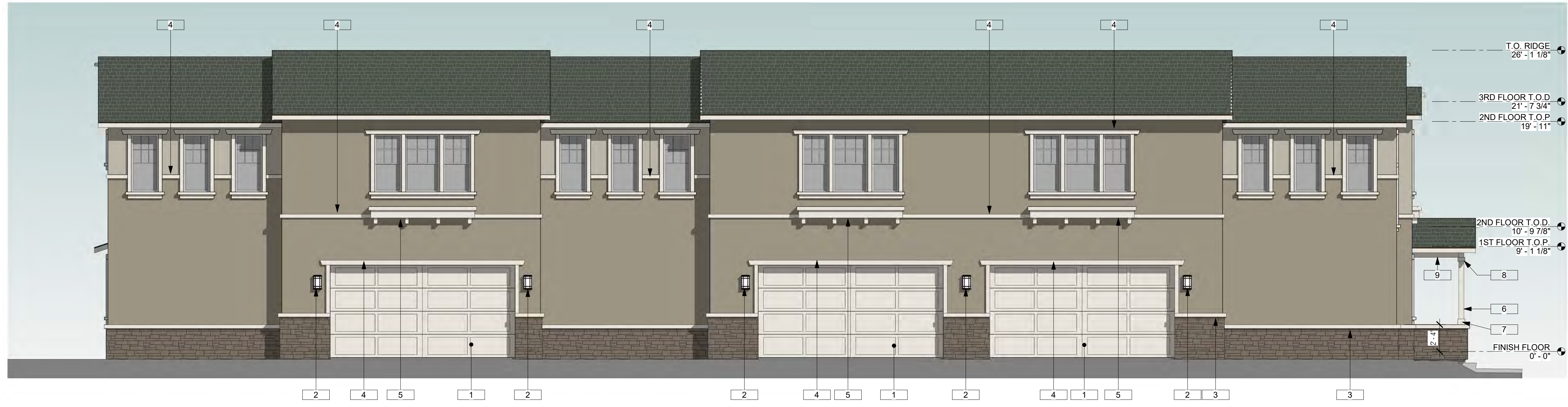
2 EXTERIOR ELEVATION B - VEHICULAR ENTRANCE SIDE 3/16" = 1'-0"
