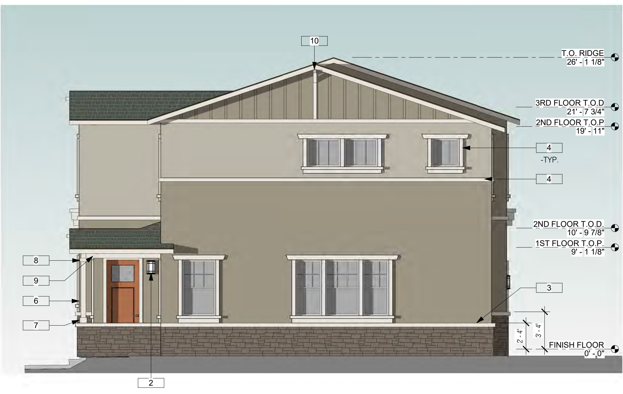
4 EXTERIOR ELEVATION B - REAR 3/16" = 1'-0"
